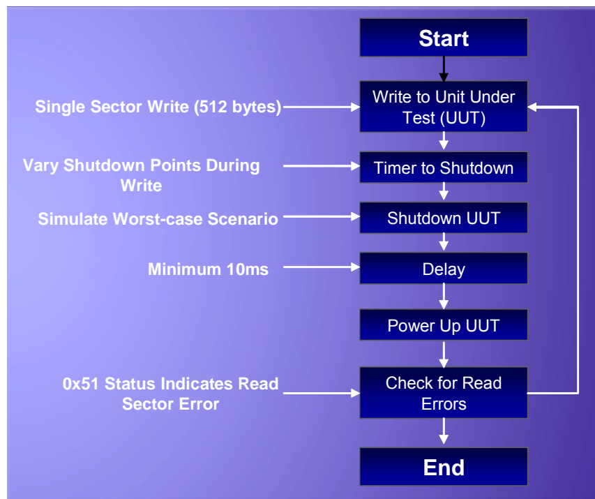
Figure 7: Sample Powerdown Test Program Flow
